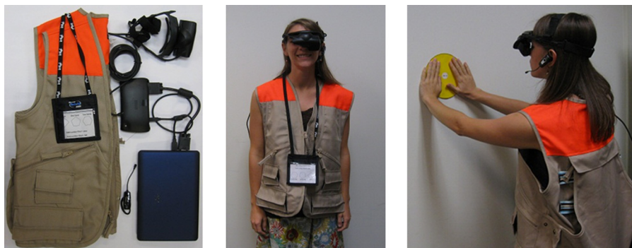
Fig. 4 (a) and (b) Monocular display hardware configuration; (c) example of a two-handed touch using the monocular display configuration
