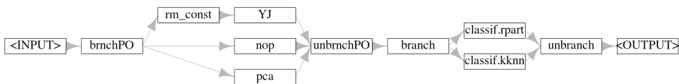
Figure 8.11: Graph with branching to three different paths that are split with po("branch") and combined with po("unbranch") then branch and recombine again.
